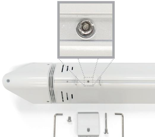
6. Once you have chosen and set the attachment position and the position of the brackets, mark the drill holes where the brackets are to be screwed to the wall or ceiling later. Hold the heater in place on the wall/ceiling to mark the drilling positions.
